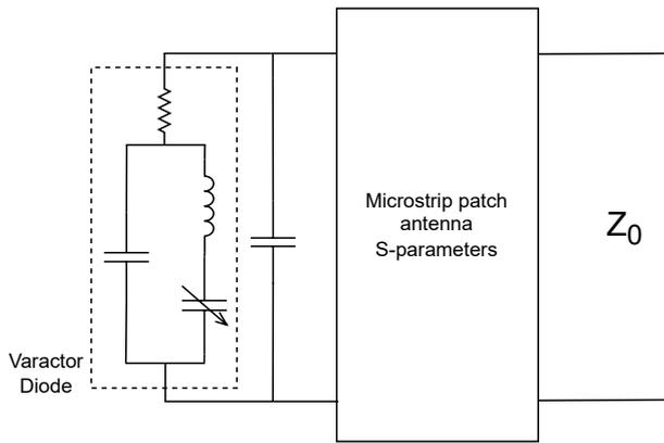
Fig. 5. Unit cell model
