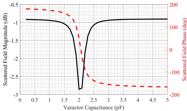
Fig. 6. Simulated reflected magnitude and phase field
