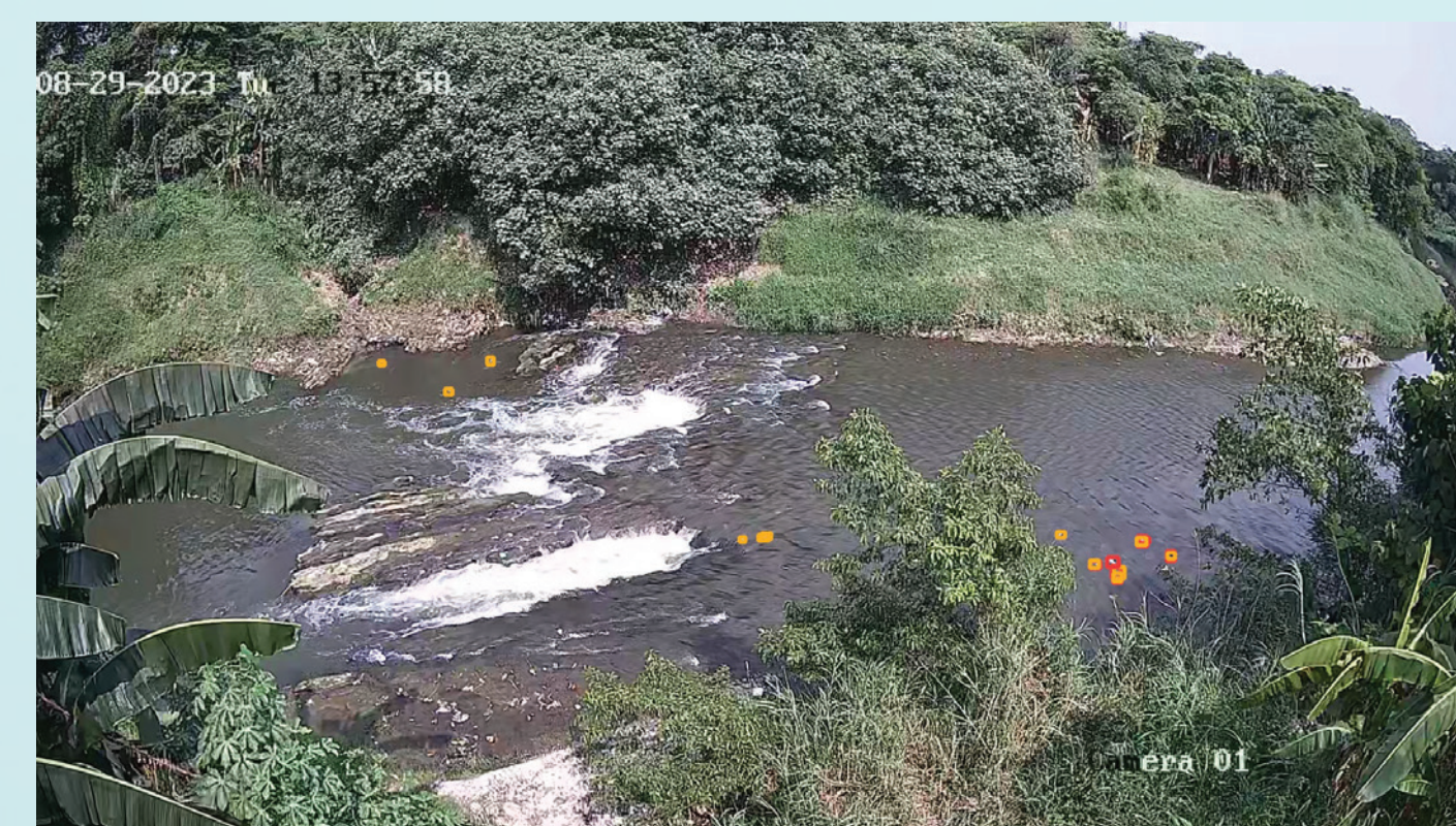
Figure 1: The data from the installed camera is downloaded and analysed in 15 minutes intervals. For the detection of floating plastic objects the CNN YOLOv5 is applied. In the figure, each detection is highlighted by an orange box.
